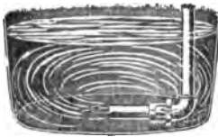
FIG. 157. —Heating Water by Steam. The arrow represents the passage of heat (by steam) into the water. The attachment is screwed onto the steam pipe.
